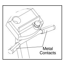
To use the pulse sensor, first make sure that the power is turned on. Stop exercising, rest both feet on the floor, and place your hands on the metal contacts. Your palms must be resting on the inner contacts and your fingers must be touching the outer contacts. Avoid moving your hands. After a moment, the heart indicator in the PULSE display will flash and your heart rate will be shown. For the most accurate heart rate reading, continue to hold the contacts for about 15 seconds.
